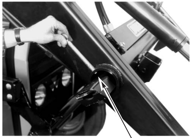
Fully Insert Stands And Pin Into Place
